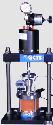
PNEUMATIC LOAD FRAME
