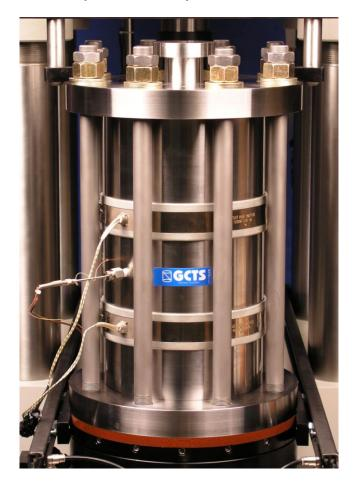
The standard cell includes 5 electrical feed-through connectors with 4 lines each (20 electrical lines total) to connect a variety of internal sensors such as deformation gages, P & S wave velocity transducers, acoustic emission sensors, etc.
