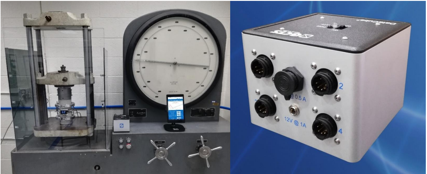
(Legacy load frame upgrade with the DataCube)
