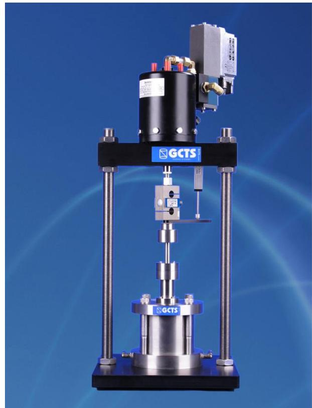
The CRS-10 system can be easily upgraded to a full triaxial test system. Consult GCTS for pricing information.
