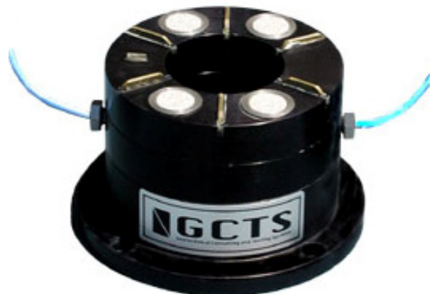
Platen for Hollow Soil Specimens with Embedded Compression Crystal and Protruding Bender Element
