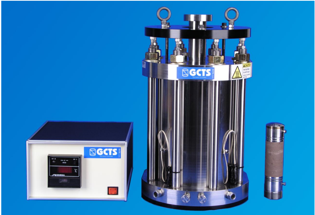
HTRX-140 with temperature control option (heaters inside cell wall) & ultrasonic platens
